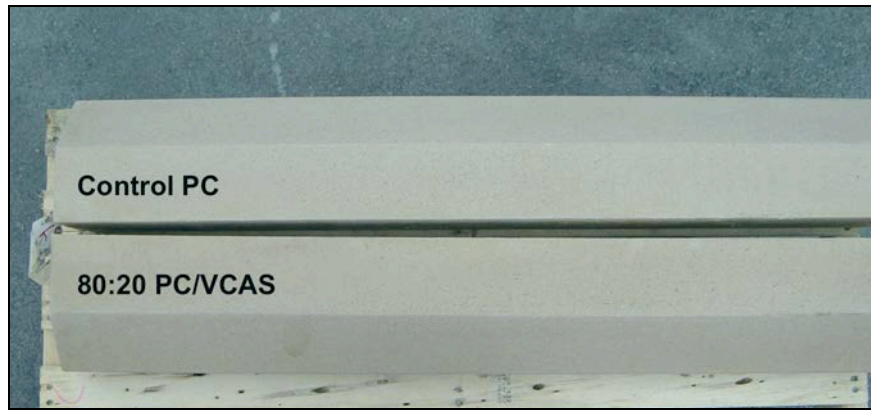
Architectural concrete beams: PC Control (top) and 80:20 PC/VCAS concrete (bottom)
