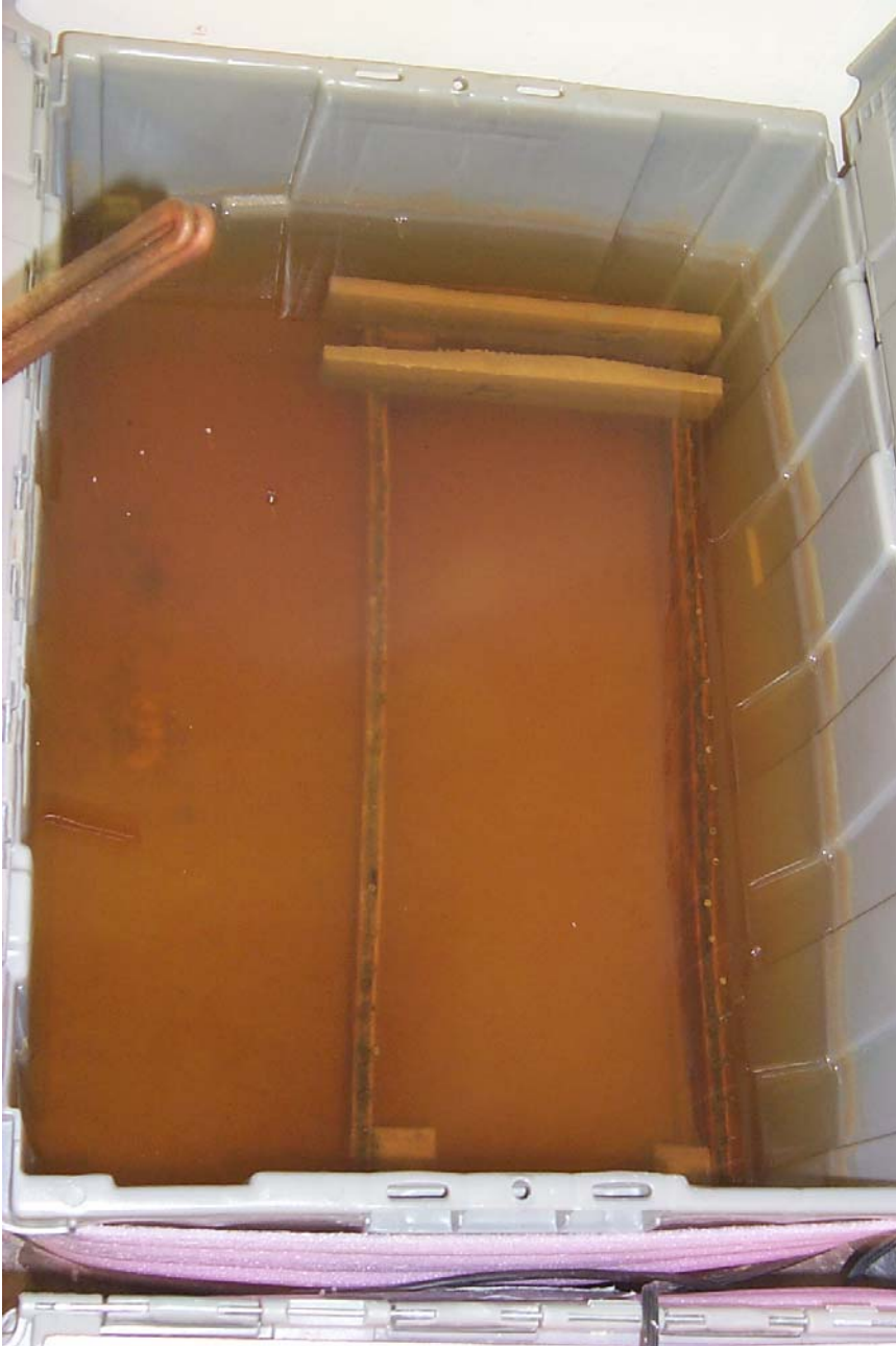
Figure 3 – Test Coupons Placed in racks inside the Hot Water Tank.
