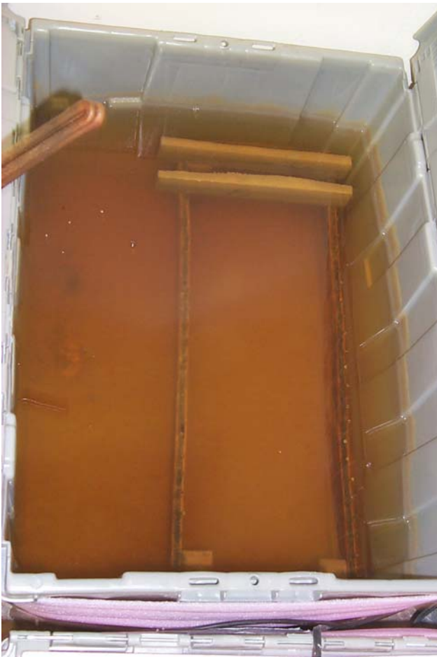
Figure 3 – Test Coupons Placed in racks inside the Hot Water Tank. Test Results
