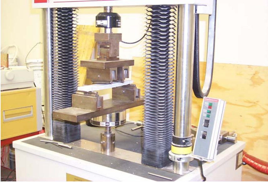
Figure 1 – Flexural Strength Test Rig
